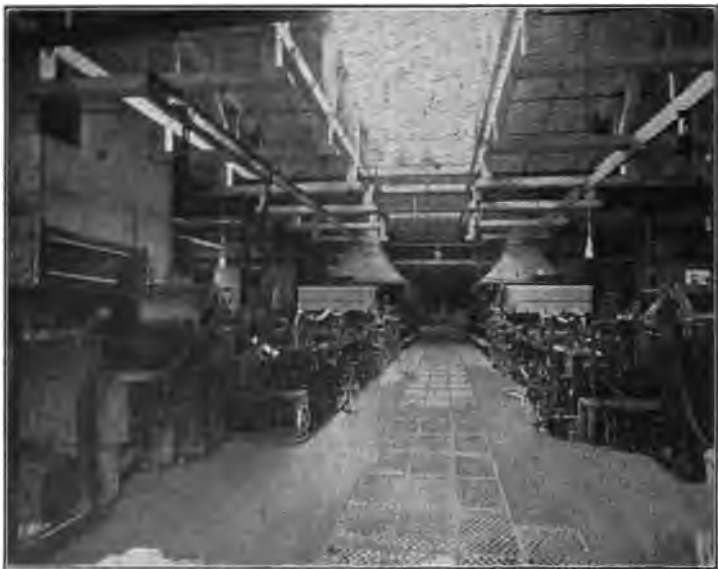
FIG. 137.—Wet end of a Fourdrinier paper machine. (Courtesy of B. D. Rising Paper Co.)
